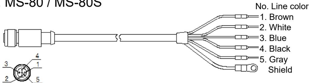
Figure 7-3. Output Cables [MS-80 / MS-80S]
