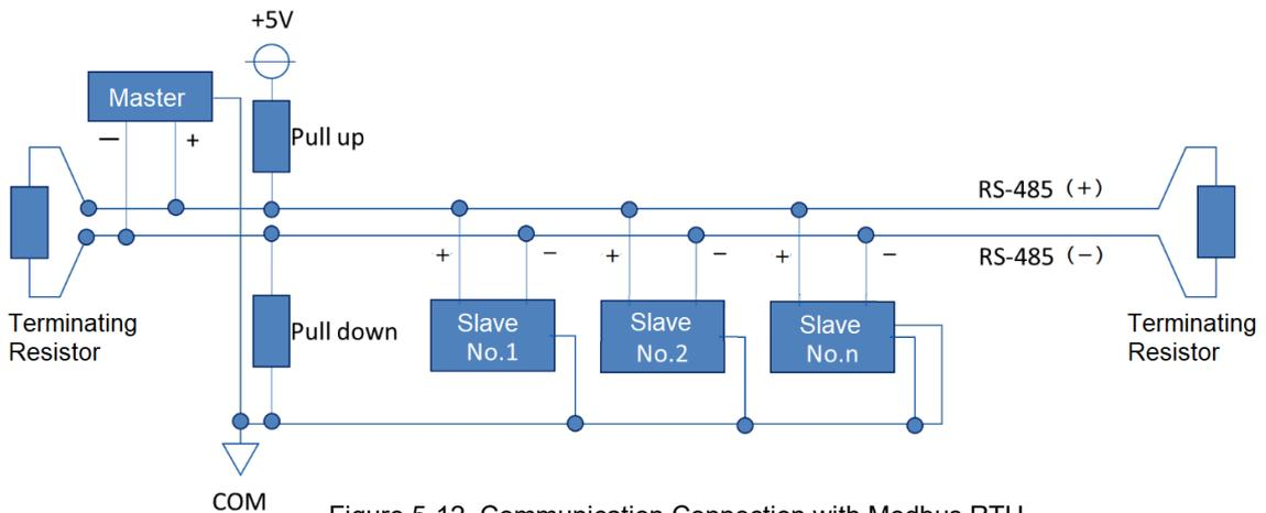
Figure 5-12. Communication Connection with Modbus RTU
