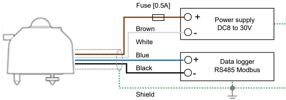
Figure 5-11. How to connect MS-80S (Modbus RTU)
