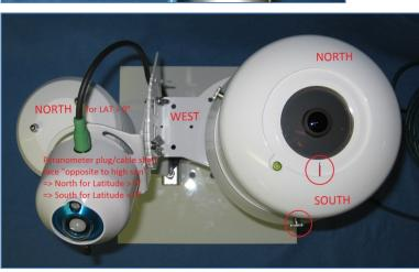
When mounting the Pyranometer, consider Northern or Southern hemisphere. The plug and cable always shall face "away from sun", to avoid heat by exposure to direct sun radiation, therefore likely corrupt Pyrano irradiance data.
