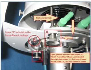
For proper mounting of the "Pyranometer Mounting Arm", follow instructions within the picture. - NOTICE: There are three possible ways of mounting. Only ONE ensures the correct North-South arm orientation, necessary for non 90° tilt angle adjustments, required for GTI.
