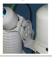
Allows very easy mounting of one Pyrano to an ASI-16 body without special additional (mechanical) tools and components.
