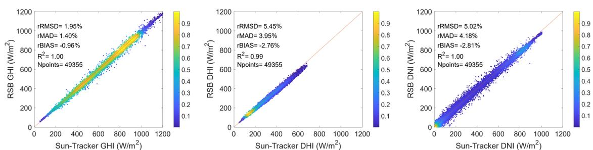
Figure 2. All Weather comparison, RSB vs. Suntracker based GHI, DHI and DNI measurements.
