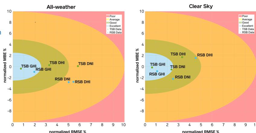
Figure 4. RSB and TSB Measurement accuracy under All-Weather and Clear Sky conditions
