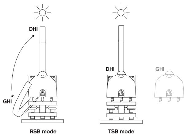
In RSB mode, the shadow band alternates between shading and unshading the pyranometer, allowing the measurement of both DHI and GHI, while calculating DNI with a single instrument. In this work, we introduce and evaluate a new operational mode called the Tracking Shadow Band (TSB) mode, where the instrument continuously measures diffuse irradiance. When combined with an additional pyranometer to measure GHI, DNI can also be determined.
