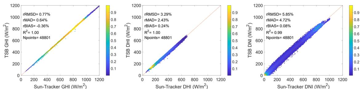
Figure 3. All Weather comparison, TSB vs. Suntracker based GHI, DHI and DNI measurements.
