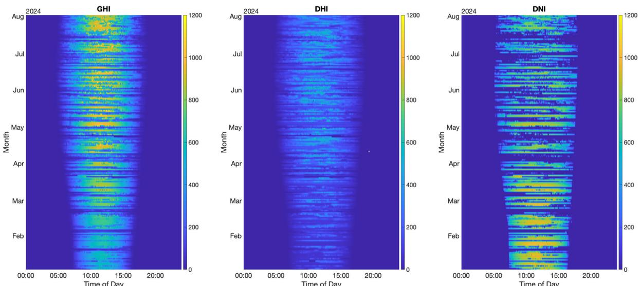
Figure 1. Reference suntracker based GHI, DHI and DNI measurements, collected from January to August 2024
