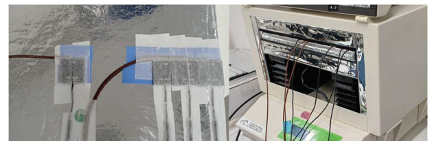
Fig.3: Installation of HF-01S on VIPs and placing in FOX314
