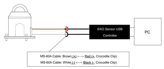
Figure A-5. Connection by EKO Sensor USB Controller
