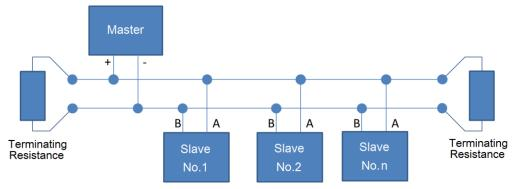
Figure 5-5. Communication Connection with Modbus RTU
