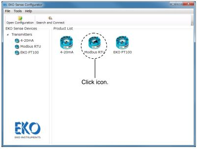
Figure A-13. Selecting Configuring Device
