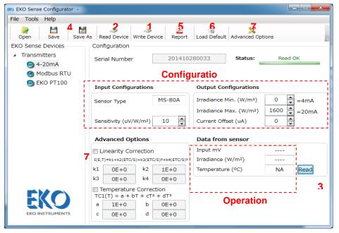
Figure A-11. EKO Sense Configurator Configuration
