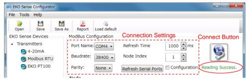
Figure A-14. MS-60M Connection Setting
