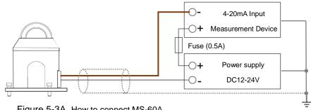
Figure 5-3A. How to connect MS-60A
