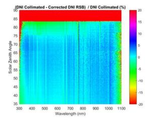
Fig. 5. DNI measurements comparison between rotating shadow band and collimation-tube configurations. DNI comparison for uncorrected DHI (left) and with corrected DHI (right)
