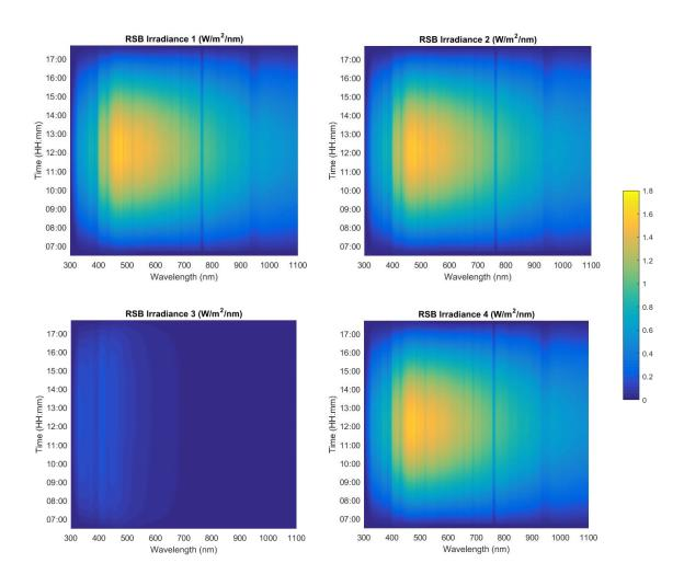
Fig. 3. RSB spectroradiometer measurements at different positions:  $1^{st}$  position GHI,  $2^{nd}$  position band at -5 °,  $3^{rd}$  position DHI,  $4^{th}$  position band at +5°
