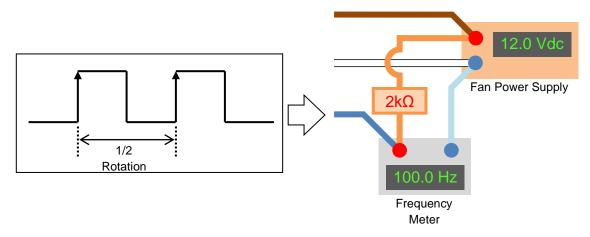
Figure 5-3. Tachometer Signal
