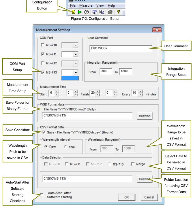
Figure 7-3. Measurement Setup Window
