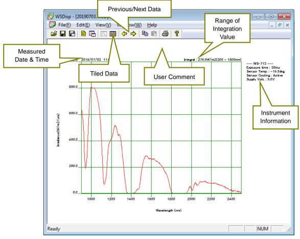
Figure 8-5. Measured Data Details Window
