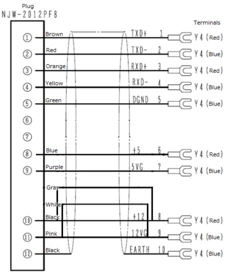
Figure 10-1. Sensor Cable Connections
