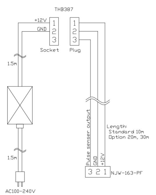
Figure 10-2. Ventilation Unit Power Supply Cable Connections
