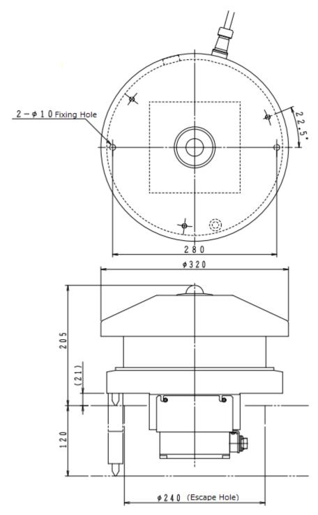
Figure 10-3. Sensor Part Dimensions
