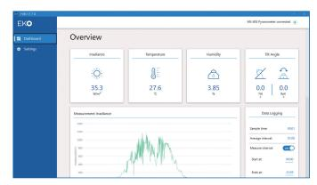
All S-Series pyranometers come with internal temperature, humidity and tilt sensors for self-diagnosis, with calibration timing and abnormality detection results visible in Hibi.
