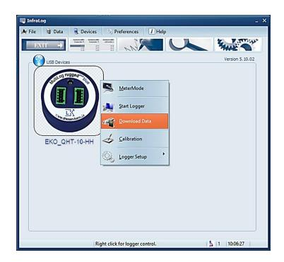
Figure 9- Click "Download Data" to download the measured data in the PC
