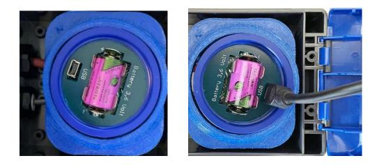
Figure 3- A round logger can be observed once the unit is opened. Locate the USB port and connect the unit to the PC using the USB port.
