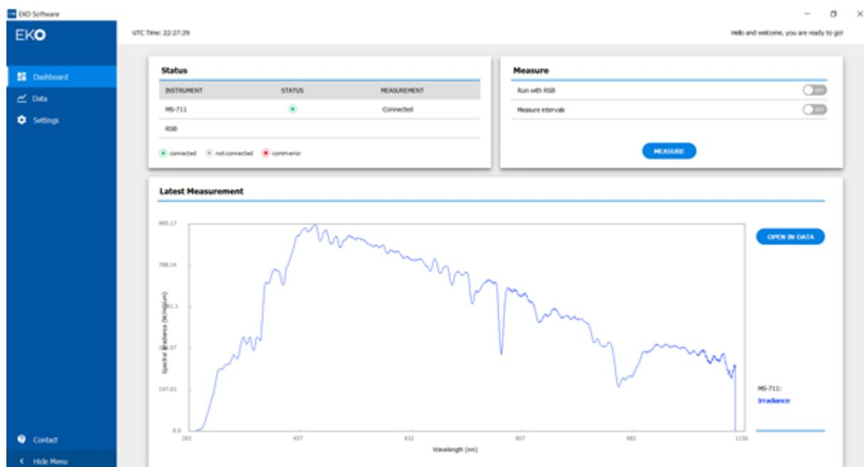
Fig.4-2-2 Basic Dashboard display with a MS-711 providing a single measurement.
