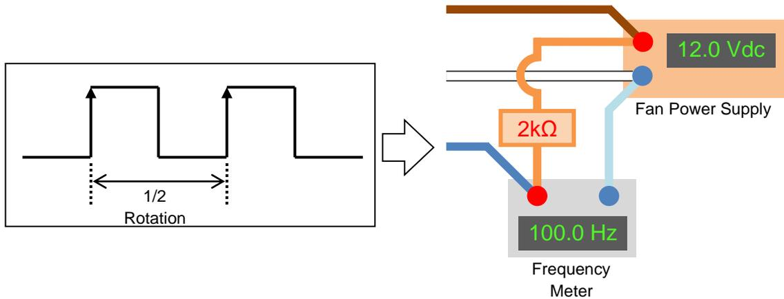
Figure 5-3. Tachometer Signal
