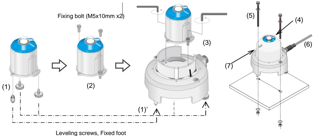
Figure 5-2. Installing the solar radiation sensor on MV-01
