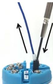
Figure 5-2. How to Remove Communication Cables
