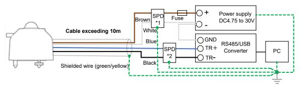
Figure A10-1. Modbus connection (when the cable length exceeds 10m, etc.)
