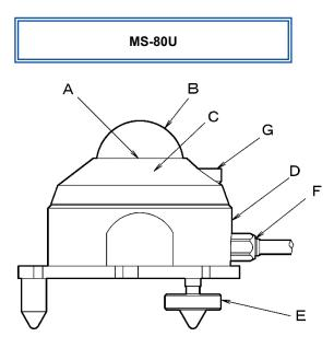
\*The cable can't be removed from the pyranometer Figure 5-2. Pyranometer Parts Name [MS-80U]
