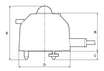
Figure 7-1. External Dimensions (MS-80/80S)
