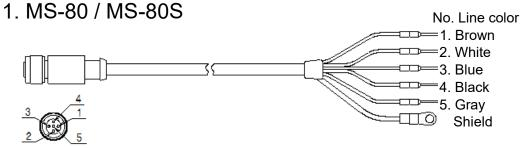
Figure 7-3. Output Cables [MS-80 / MS-80S]
