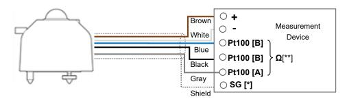
Figure 5-5. How to connect MS-80 (from S/N: S1904615)
