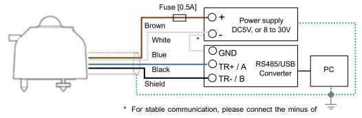
the power supply and the GND of RS485/USB converter.
