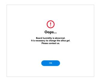
Figure A3-23. Sensor internal humidity abnormality alert
