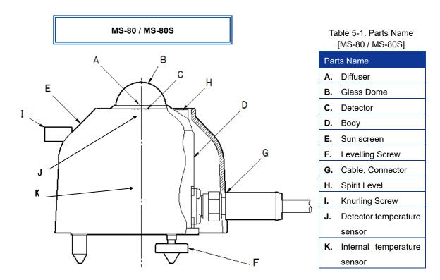
\*Signal converter is built-in for MS-80S. Figure 5-1. Pyranometer Parts Name [MS-80 / 80S]
