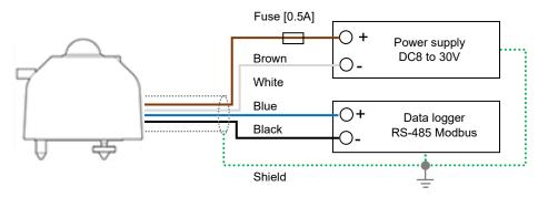
Figure 5-11. How to connect MS-80S (Modbus RS-485)
