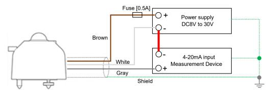
Figure 5-8. How to connect MS-80S (4-20mA output)
