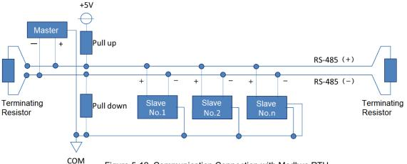
Figure 5-12. Communication Connection with Modbus RTU
