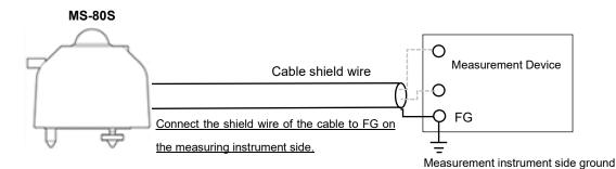
Figure 5-4B. MS-80S ground connection method
