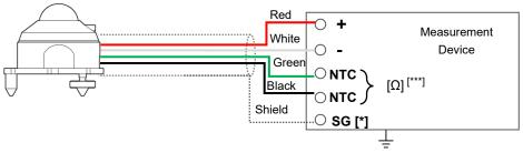
Figure 5-7. How to connect MS-80U
