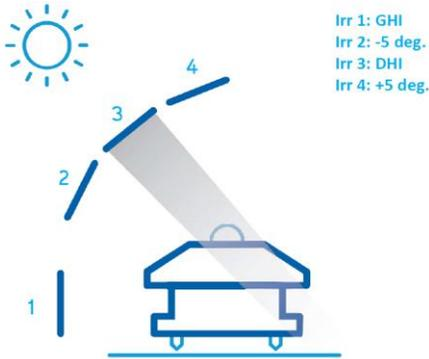
Fig. 2. Rotating shadow band sweeping positions
