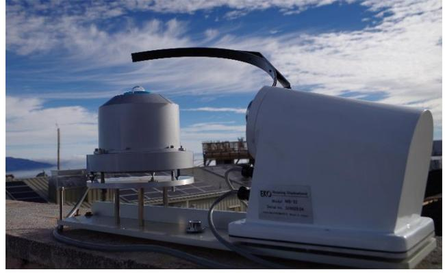
Fig. 1. Left: MS-700, MS-710, MS-711 and MS-712 mounted on an EKO STR-32G tracker; Right: EKO MS-711 mounted with the RSB-01S rotating shadowband.
