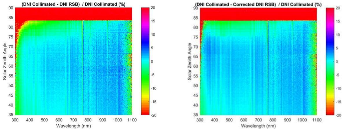
Fig. 5. DNI measurements comparison between rotating shadow band and collimation-tube configurations. DNI comparison for uncorrected DHI (left) and with corrected DHI (right)
