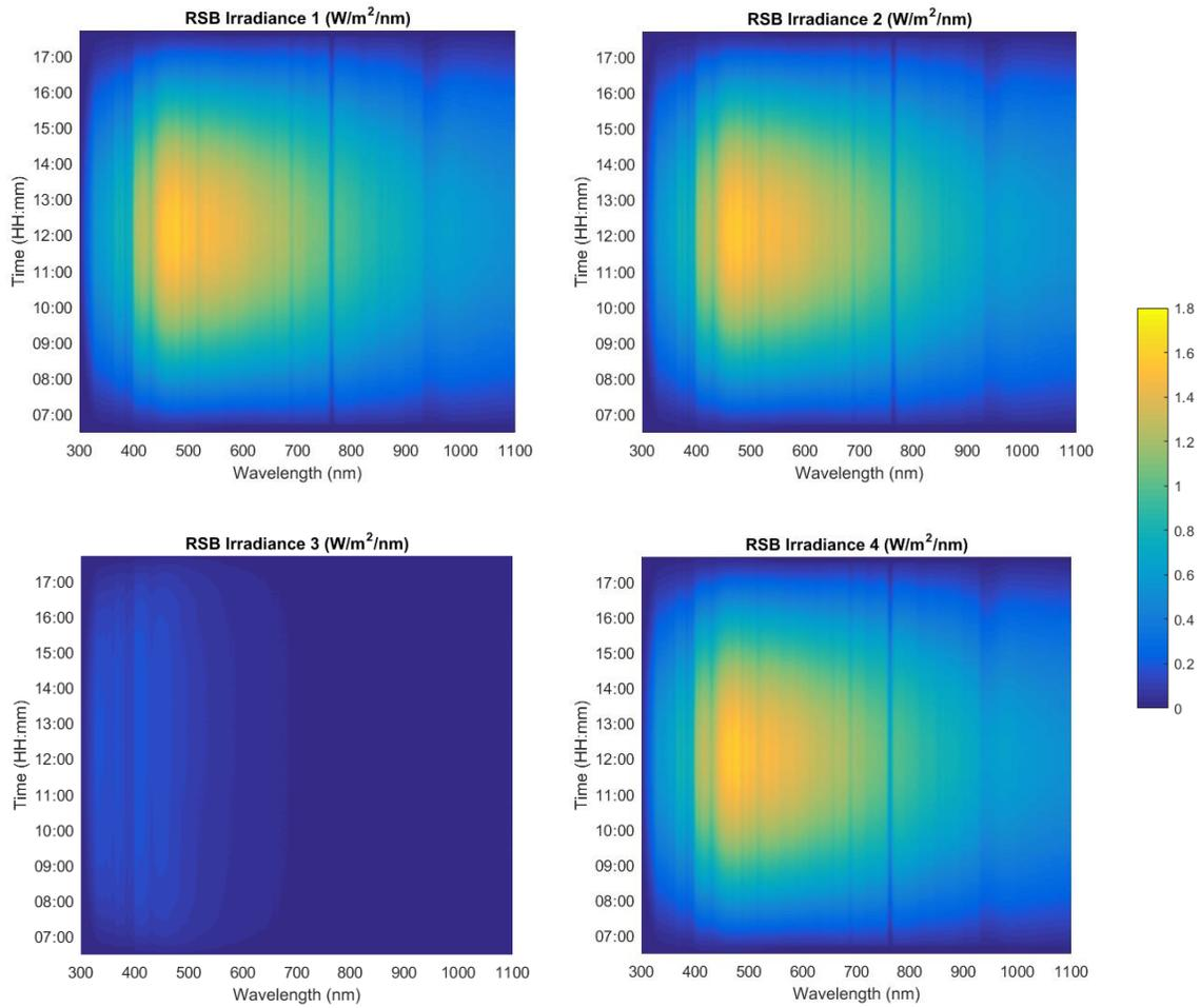
Fig. 3. RSB spectroradiometer measurements at different positions: 1<sup>st</sup> position GHI, 2<sup>nd</sup> position band at  $-5^\circ$ , 3<sup>rd</sup> position DHI, 4<sup>th</sup> position band at  $+5^\circ$
