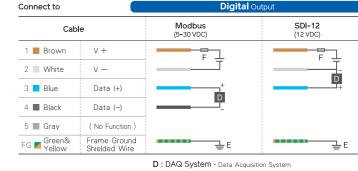
F: Fuse (0.5A) - Connect in series between power supply lines. E: Earth Connection - Be sure to connect it to the ground
