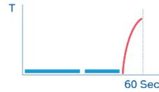
When there is a large heat loss, the sample surface temperature is low
