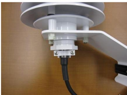
Figure 4-5. Insert Temperature Sensor
