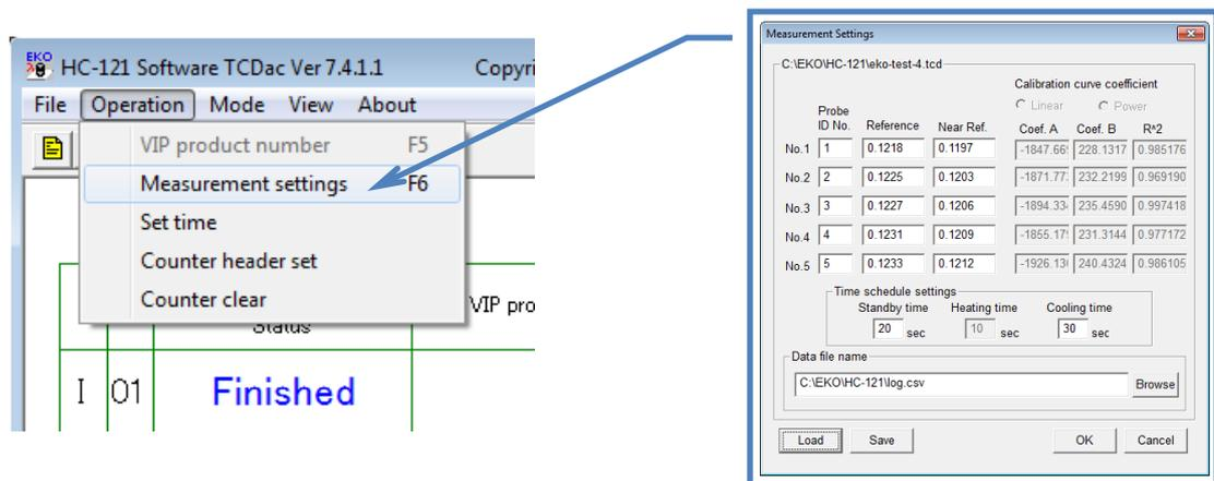
Figure 6-35. Operation Menu & Measurement Setup Display
