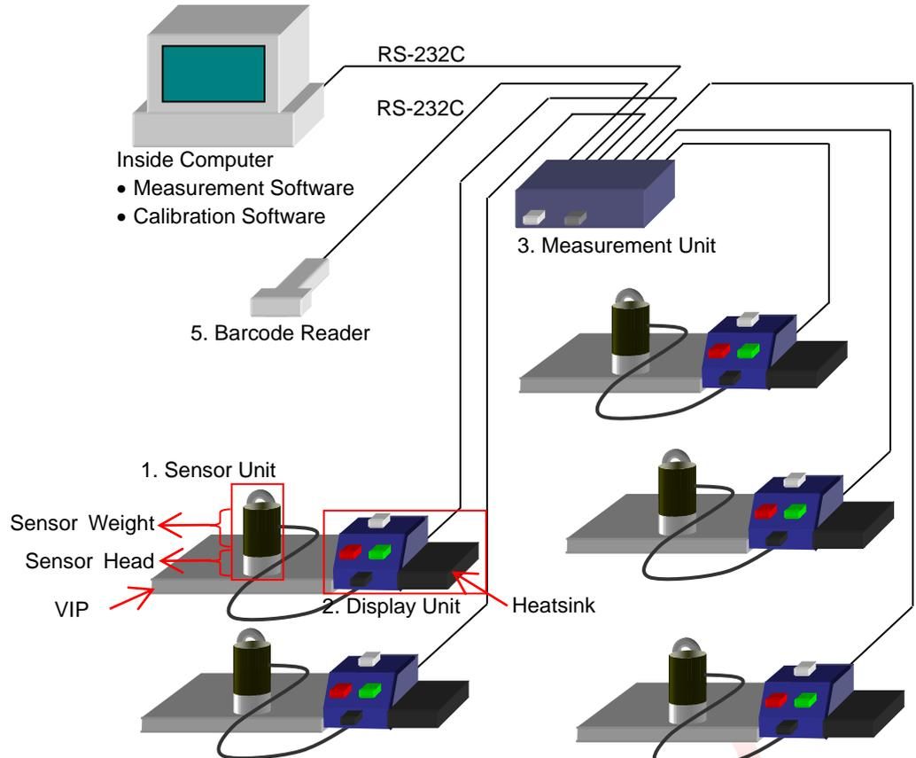
Figure 5-1 VIP Checker HC-121 System Configuration
