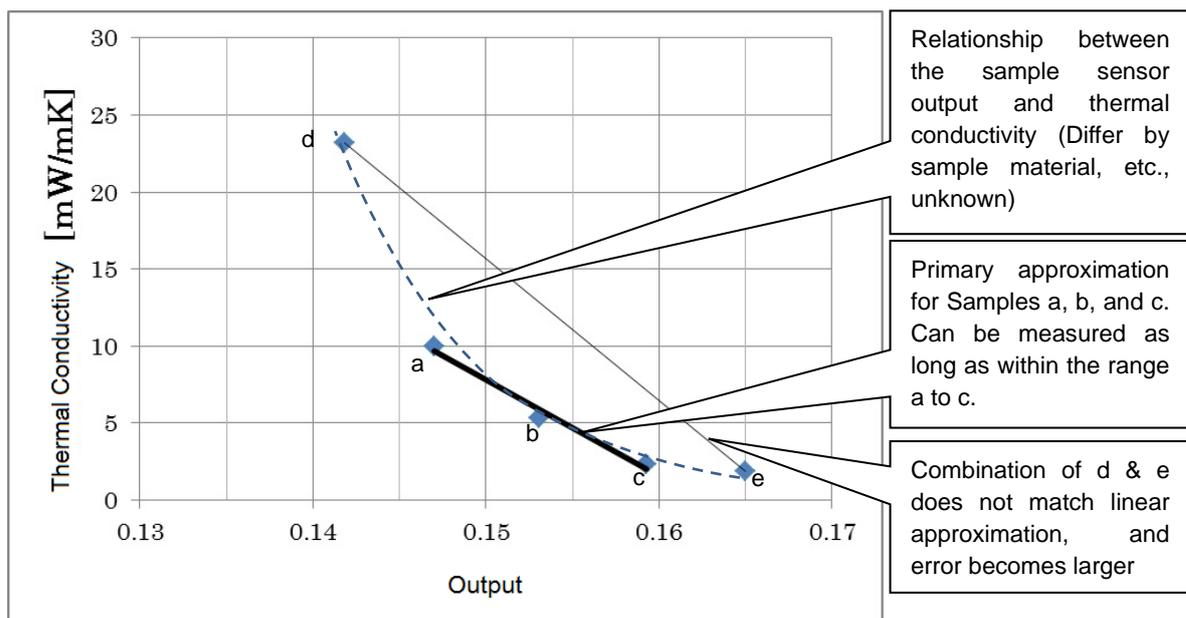
Figure 6-13a. Calibration Curve by Linear Approximation
