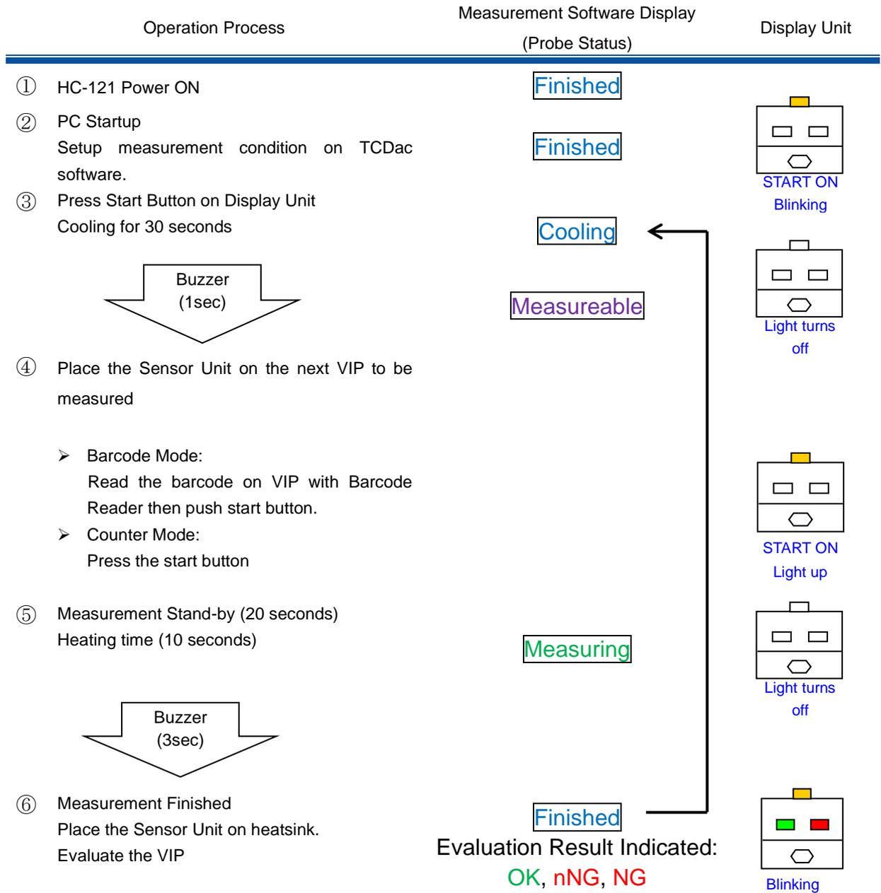
When the start button is blinking, place the Sensor Unit on the heatsink and press the start button; the process will go back to the step ③ to start cooling and the measurement can be continued repeatedly.
