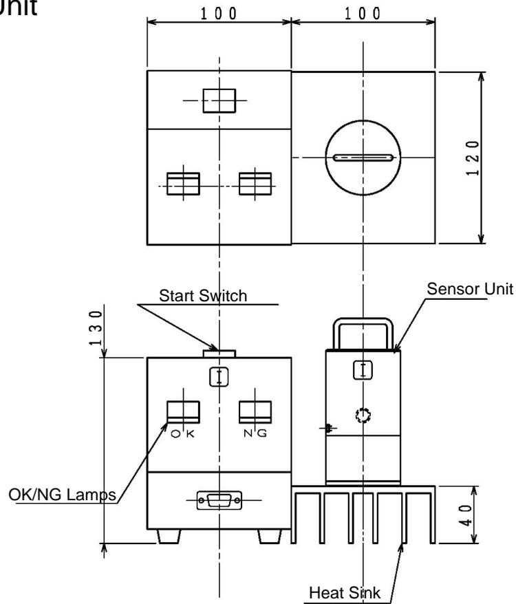
Figure 9-2. Display Unit Dimension
