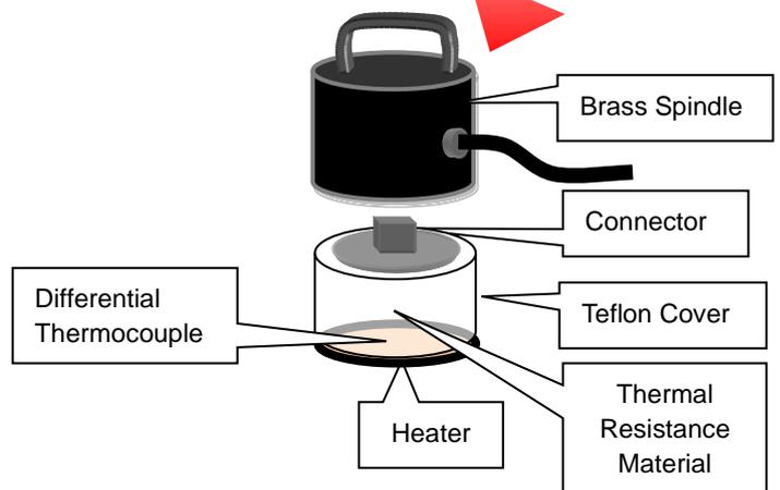
Figure 5-2. Sensor Unit Configuration
