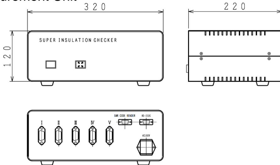
Figure 9-1. Measurement Unit Dimension
