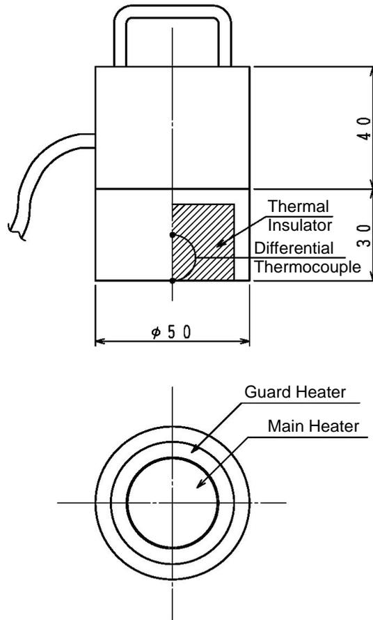
Figure 9-3. Sensor Unit Dimension
