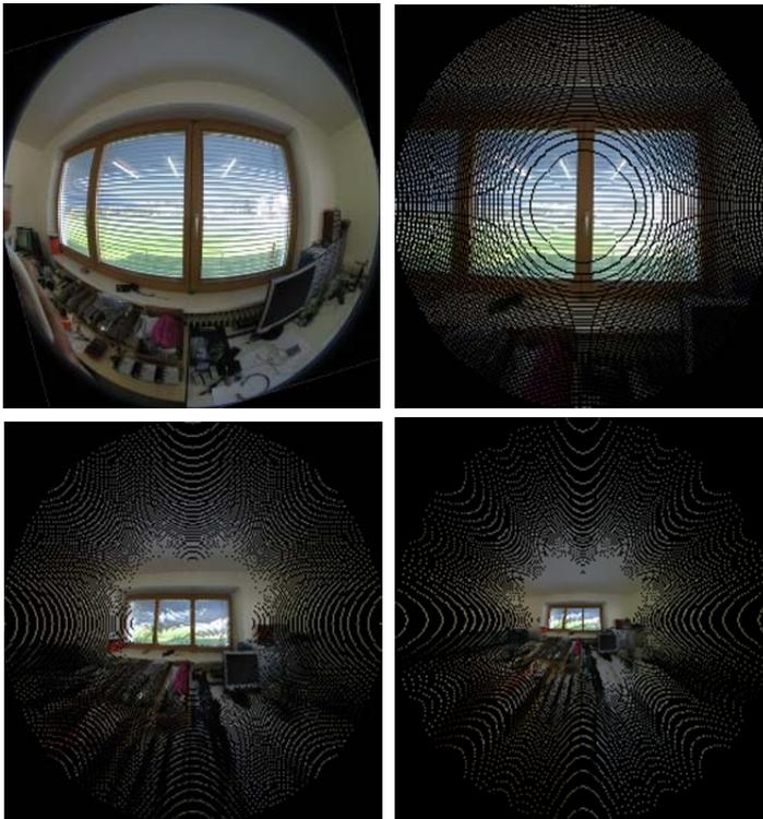
First image is original fisheye lens image, second is projection of  $60^\circ$ , third of  $80^\circ$  and fourth of  $85^\circ$ .
