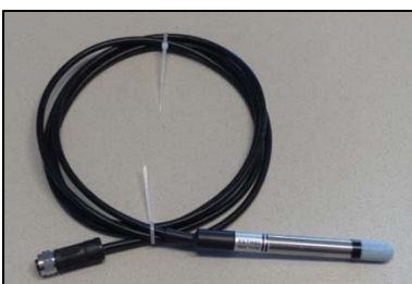
(a) External T/RH (Temperature - Humidity) Sensor:
